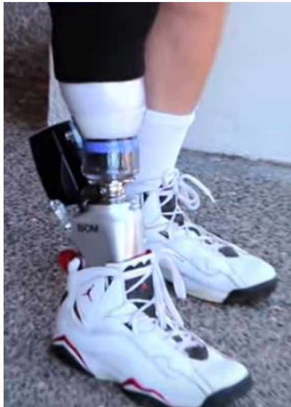
Figure 1. Image of a prosthetic leg using a BiOM [6]
