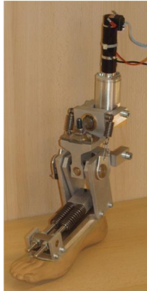
Figure 15. Ankle Prosthesis prototype developed by UCL-Belgium [3]
